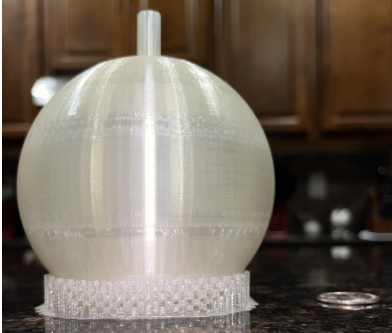
Figure 28: PLA print of the "innovative" PV. The material at the bottom is a support structure added during the build to prevent deformation.
