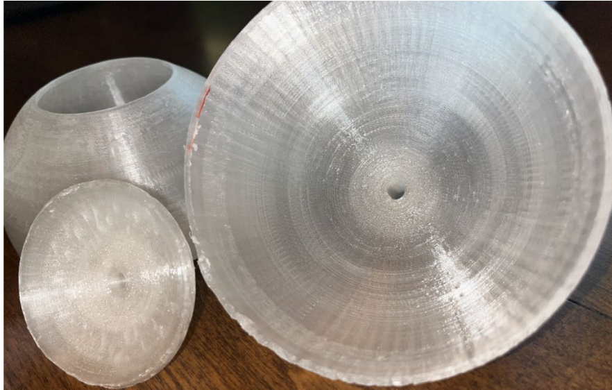
Figure 54: Article for the "innovative" model cut in half for visual inspection.
