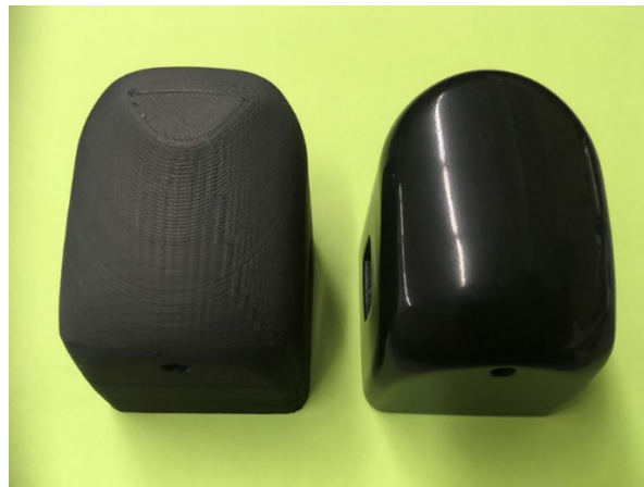
Figure 9: Example of a PLA part that has been surface finished by dry-tumbling with hardwood medium. (Steven Schneider, Kramer Industries, Inc., Vibratory Tumbling 3D Printed Plastic and Metal Parts | Kramer Industries, Inc (kramerindustriesonline.com) )
