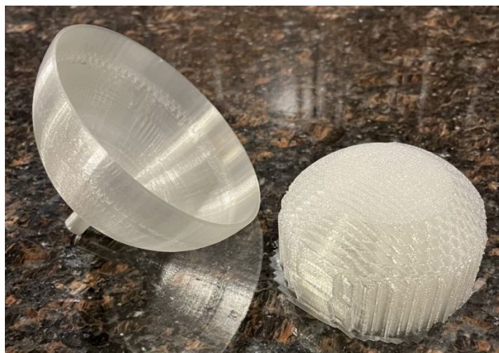
Figure 25: PLA print of the hemisphere showing the support structure removed.
