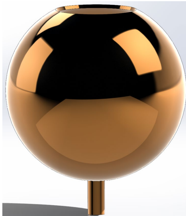
Figure 17: Sketch revolved around the axis to produce a 3D major body piece.
