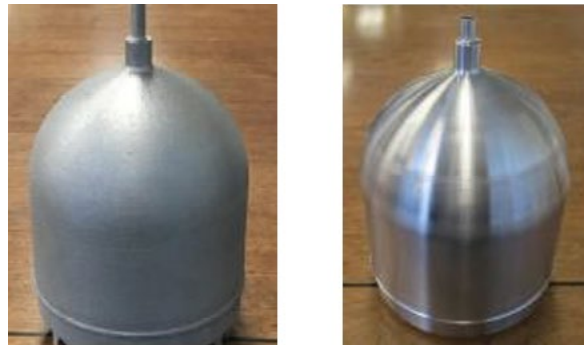
Figure 7: Two AM produced pressure vessel parts manufactured by NGIS. The left artifact has had no surface postprocessing work. The artifact on the right has undergone machining, giving it a shiny finish. (ASME, https://doi-org.ezproxy.lib.ou.edu/10.1115/PVP2019-94033 )
