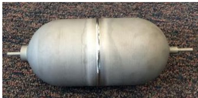
Figure 8: An AM produced pressure vessel manufactured by NGIS. This article is a cylindrical PV with spherical ends. Note the location of the weldment at the midpoint of the cylinder.(ASME, https://doi-org.ezproxy.lib.ou.edu/10.1115/PVP2019-94033 )
